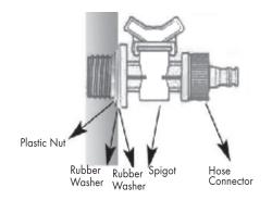
Reattach the rubber washer first and then the plastic nut from the inside of the Rain Barrel to secure the spigot in place.
