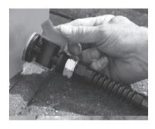
Open or close the spigot by turning the red thumb screw counter-clockwise to open and clockwise to close
