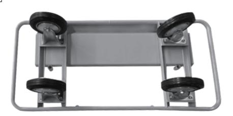
Assemble two casters and two figid wheels on bed with M8\*16 bolt, washer and lock nut, tighten.
