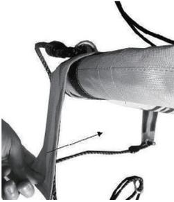
After the bolts are assembled, cover the hook and loop fastener belt, and repeat the installation of the other 3 bolts 3 times.
