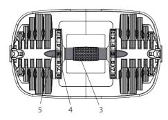
4. Push back Pin boxes (2) on both sides, and make sure Lock buttons (1) in safe lock status.
