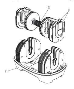
**NOTE:**Because PA material itself has the characteristics of water absorption expansion (including moisture in the air), pin box and other components may absorb water and cause the problem of shrinkage of fit clearance.
