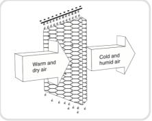
The recommended relative humidity for optimum operation is 60% or lower. A drier climate makes for more noticeable cooling.
