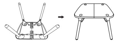
4. Connect the seat and the desktop board according to the corresponding number, press the middle part of the seat to click into the desktop, then install the dinner plate, and the dining chair is installed.
