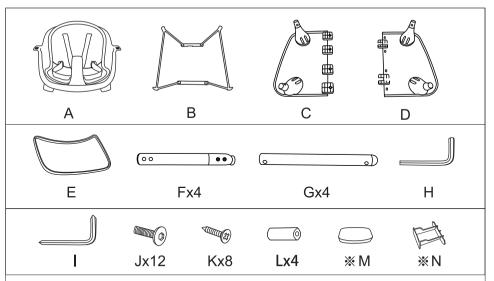
(A)Seat (B)Desktop holder (C)Desktop left (D)Desktop right (E)Dinner plate (F)Upper seat legs (G)Lower seat legs (H)Hex wrench (I)Cross wrench (J)M6\*25Bolts (K)M5\*15Self-tapping screws (L)Pad tube
