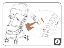
4 Press the small button on the armrest plug as shown, then lift it up to remove the armrest. Insert the armrest plug into the armrest socket of the frame when installing.
