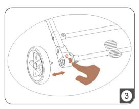
3 The rear wheel can be disassembled by pressing the quick disassembly button "e" as shown in the figure. When installing the rear wheel, it is only necessary to insert the rear wheel in the direction shown in the figure.
