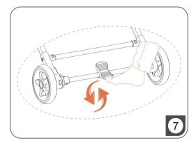
7 Press the brake pedal forwards to lock the wheel, press it backward to unlock the wheel.
