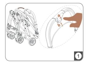
1 Press the safety button "a" as shown in the figure, then pinch the "b" of the pick-up button, then press down the push handle to make it fold. Expansion is the reverse process of folding up.
