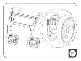
2 The front wheel can be removed by pressing the front wheel quick disassembly button "c" as shown in the figure. When installing the front wheel, it is only necessary to insert the front wheel in the graphic direction. The front wheel orientation can be achieved by pulling up and down the orientation button "d".
