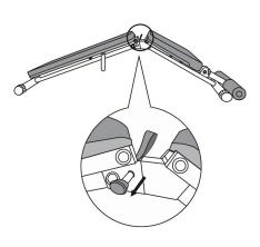
2. Take Part#C out from the backrest, seat and foot rack, and fold as below, then insert Part B to lock the bench as the following picture.
