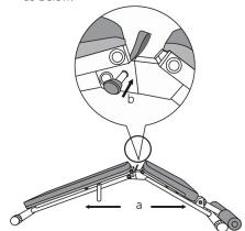
③ Adjust the backrest, seat and foot rack to your needed position and insert Part# C into the adjustable fixing hole as below. ④ Put felt mat under support feet as below.
