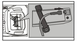
7.Connect the power As showed in the picture, connect the motor plug -in with the car, then connect the power plug-in with the right direction.
