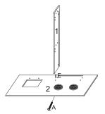
Insert E (wooden dowel) to No.1 panel, use A screw to lock it on No.2 panel.
