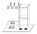
Use B screws to lock No.35(3pcs) on No.3 panel, use C screws to lock taps(O) on counter-table.
