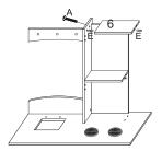
Insert E(wooden dowels) to No.6 panel, use A screw to lock it on No.1 panel.
