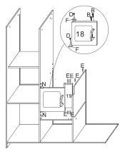
Insert N( hinges) on No.18 panel, insert E (wooden dowel) to No.19 and No.17 panel, use B screw to lock J( handle) on No.18 panel, use D screw lock F(hinges) on No.18 up and down.
