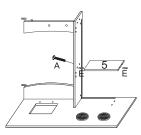
Insert E(wooden dowels) to No.5 panel, use A screw to lock it on No.1 panel.
