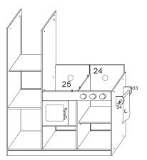
Put inside No.24 and No.25 panel in groove, insert L(bar) to No.33 and No.34 panel.
