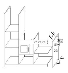
Insert E(wooden dowels) to No.32 panel, use A screws to lock it on No.23 panel, use A screws to lock No.23 panel to No.11 panel.
