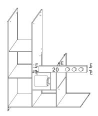
Insert E(wooden dowels) to No.20 panel.
