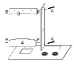
Insert E(wooden dowels) to No.3 and No.4 panel, use A screws to lock it on No.1 panel.
