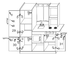
Use B screws to lock I(handles) on No.29,30 and 31 panel, use D screw lock the female(3 pcs) door latches on No.16 and 17 panel, use D screw lock the male(3 pcs) door latches on No.29,30,31 panel, use D screw lock hinges on No.29, 30,31 panel.
