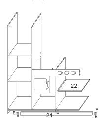
Insert E(wooden dowels) to No.21 panel, insert No.22 panel to No.17 panel groove.
