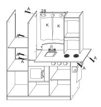
Put the upper finished parts on kitchen, use A screws to lock it on kitchen, put K (fabrics) inside No.28 (bar).
