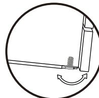
3.1 Place the dishwasher levelly in case of triggering overflowing and electricity leakage. The ventilator showed in the figure should not be placed on the rug.
