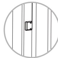
① Remove the lid on both sides of the appliance for putting screws on them.
