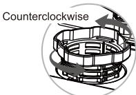
1. Rotate the filter cup counterclockwise to remove the filter cup.
