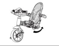
4.Lift the main frame body back and open it as shown in the picture.
