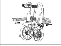
3. Open the guardrail as shown in the picture.
