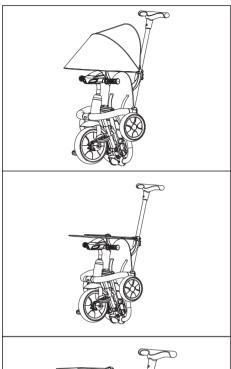
4.Lock the guardrail as shown in the picture.
