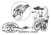
2.Install 1.5V\*3 battery on the music box and fix the battery cover, as shown in the picture. Then install the front music box on the handlebar and tighten it with 4 tapping screws of ST3.5 \*15.
