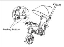
2.Press the folding button to fold the rear frame forward and up (until you hear "Click" sound).
