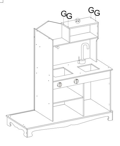
STEP 17: Assemble No.22 to No.20 and No.17 with screws G.
