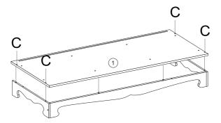
STEP 6: Assemble No.1 to No.2,3,4 with screws C.
