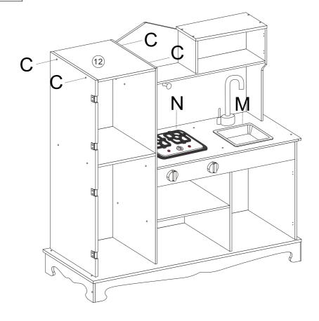
STEP 22: Assemble No.12 to No.5 and No.6 with screws C. Put parts N and M above No.15.
