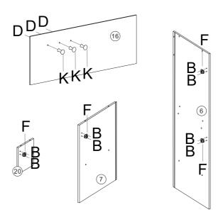
STEP 4: Assemble parts K to No.16 with screws D. Assemble parts F to No.6,7 ,20 with screws B.
