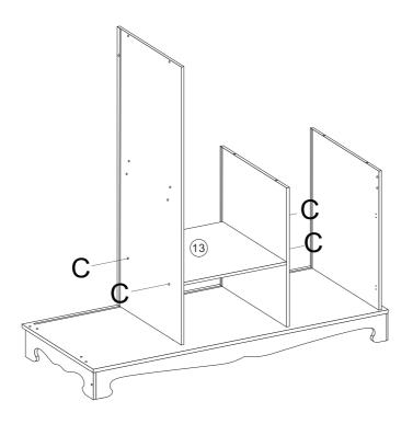
STEP 8: Assemble No.13 to No.6 and No.7 with screws C.
