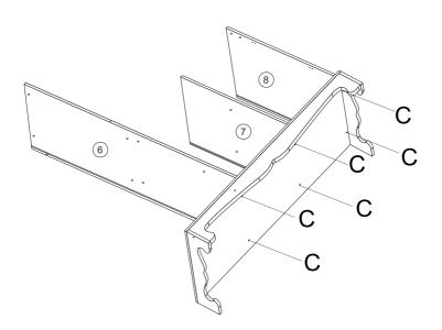
STEP 7: Assemble No.6,7 ,8 to No.1 with screws C.
