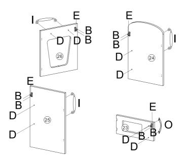
STEP 2: Assemble parts E to No.23,24,25,26 with screws B. Also assemble parts I to No.24,25,26 with screws D. Assemble part O to No.23 with screws D.
