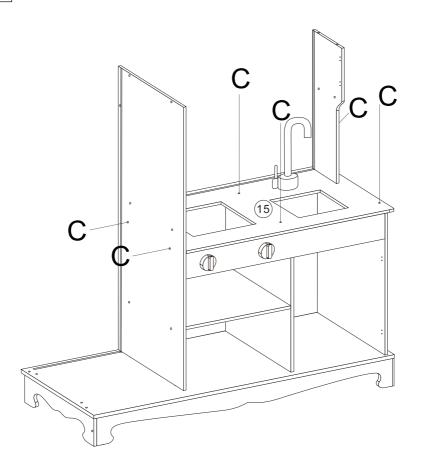
STEP 12: Assemble No.15 to No.6,7,8 with screws C.
