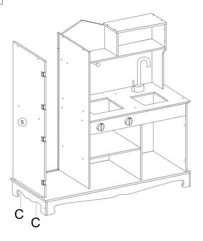
STEP 18: Assemble No.5 to No.1 with screws C.
