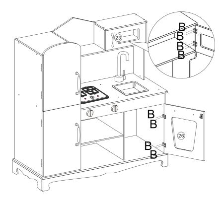
STEP 24: Assemble No.23 to No.17 with screws B, also assemble No.26 to No.8 with screws B.
