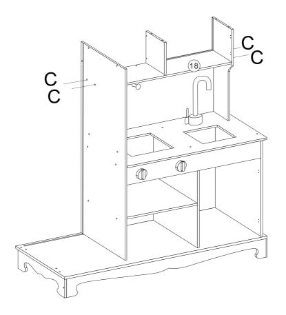
STEP 14: Assemble No.18 to No.6 and No.17 with screws C.
