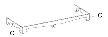
STEP 5: Attach No.2,3 to No.4 with screws C.
