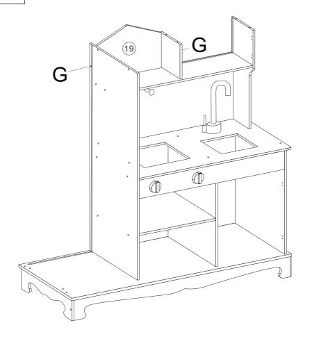
STEP 15: Assemble No.19 to No.6 and No.20 with screws G.
