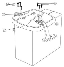
4 Note: Align the arm with the mechanism in the correct direction, referring to the FRONT label on the bottom of the seat cushion. Tighten the screws completely.
