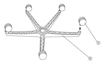
2 Select a smooth surface to avoid scratching the parts. Turn the star base upside down. Press the casters into holes at the end of each leg. Turn the star base upright and insert gas lift with telescoping cover into the central hole of the star base.
