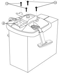
6 Connect the back cushion to the seat cushion Align the back cushion with the seat cushion and attach the back support plate onto the bottom of the seat cushion by using screws and tighten up.
