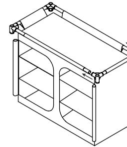
Connect the short tube, then connect the two longer tubes, finally connect the other short tube.
