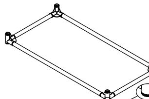
Connect the F accessory to the tubes in the same way to make the base support.
