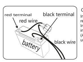
Connecting Battery Line Inserting red wire on the car into red column on the battery. Inserting black wire on the car into black column on the battery. (Avoiding inserting into the uncorrect polarity)
