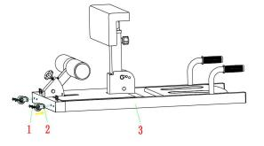
STEP 3: Assemble the wheels accessory to main frame part 3 and fix by screws
