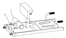
STEP 4: Adjust the height of part 2 which is suitable for your feet and fix by Knob part 8
