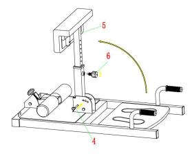
STEP 2: put part 5 on Vertical and fixed by knob part 6. Insert the pin part 4 to the suitable holes you prefer and adjust the height of backrest part 5 by knob
