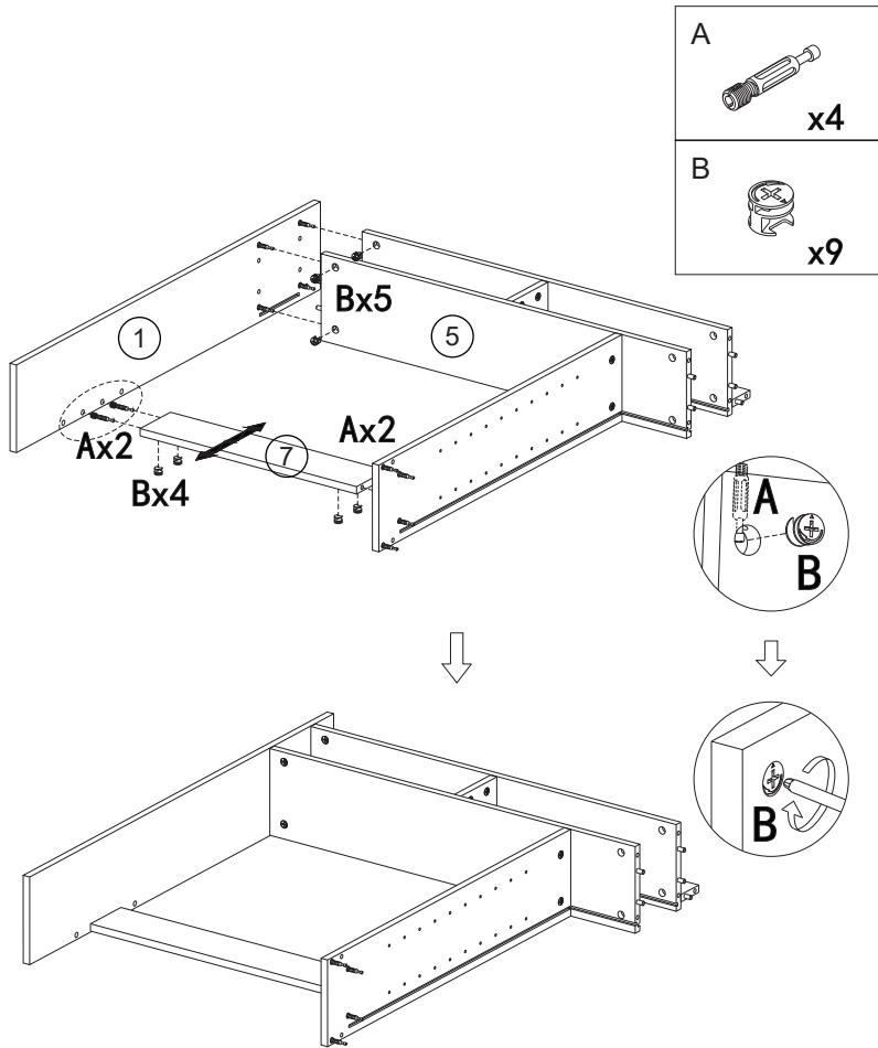
EN: There are two installation positions, which can be installed according to the height you need.
