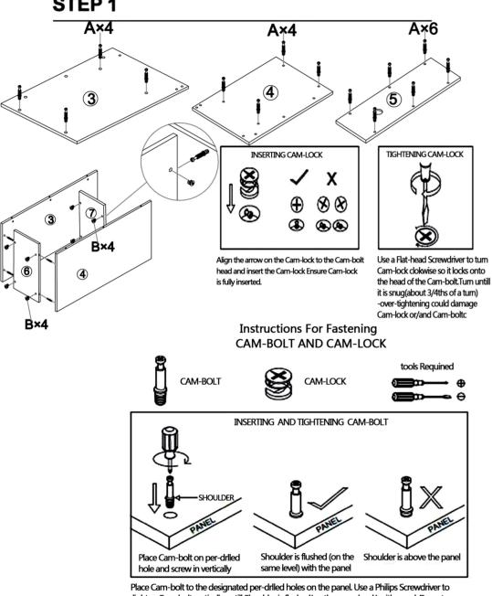
lighten Cam-bolt vertically untill Shoulder is flushed (on the same level ) with panel. Do not over-tighten or under-tighten
