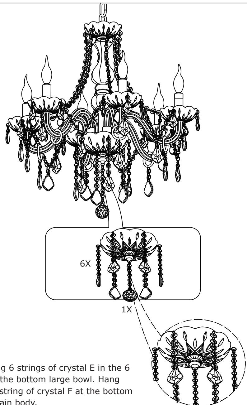
First hang 6 strings of crystal E in the 6 holes of the bottom large bowl. Hang another string of crystal F at the bottom of the main body.
