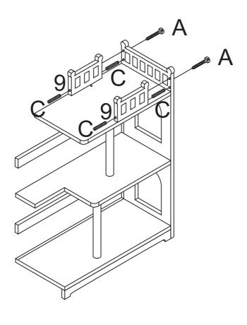
STEP 6: Assemble Part.10 to Part.8,9 with screws A.
