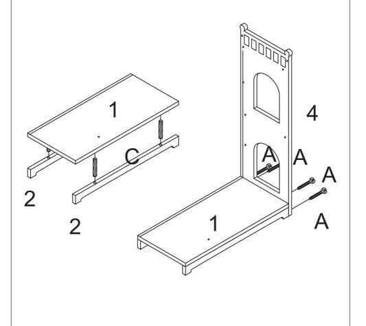
STEP 2: Assemble Part.6 to Part.1 with screws A. Assemble Part.5 to Part.4 with screws A.
