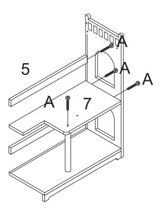
STEP 4: Assemble Part.6 to Part.7,8 with screws A. Assemble Part.8 to Part.4 with screws A.
