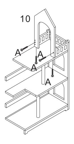
STEP 7: Assemble Part.11 to Part.10 with screws A,dowel C. Insert Part.12 to Part.1,5,7,8,11.
