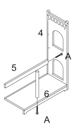
STEP 3: Assemble Part.7 to Part.6,4 with screws A. Assemble Part.5 to Part.4 with screws A.
