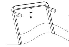
1. Place the safety lock on the yellow label of the electronic meter .As shown in illustration.
