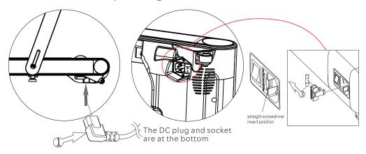
Pull out the power plug from power socket as shown in the step1 of left picture. Remove the safety socket from the power socket with a straight screwdriver as shown in the step2 of left picture. Take out the fuse according to the direction shown in the picture, and insert it after replacing it.
