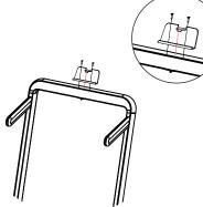
1、Fix "phone bracket" with two pieces ST4.2\*22 bolts on riser beam.
