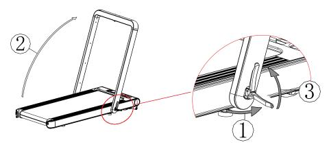
As shown in the step1 of the picture. Open the folding handle in the direction shown in the picture. meanwhile the lower end of the riser will naturally expand to the two sides. Raise the riser upward to the upper limit position as shown in the step2 of the left picture. Press "folding handle" and locked riser as shown in the step3 of the left picture.
