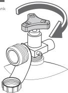
Attach fuel hose regulator to the output of the tank by turning the coupling nut clockwise.
