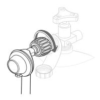
Turn release valve on tank counterclockwise to release gas.
