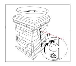
Turn the cylinder valve on the tank clockwise to close the propane tank. Attach the preassembled regulator from the Body (1) to the cylinder valve by turning the regulator coupling nut clockwise. Make sure it is fastened securely and tighten connections by hand only.
