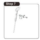
Assemble the cup holder with a screw by a screwdriver(not included).
