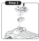
Pass the straight end of the J-shaped stick through the safety bar fixing part and align it with the hole on the steering wheel, then fix and tighten with the screw and nut.
