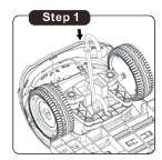
Insert the J-shaped stick into the front of the body,make sure it is in the correct position as shown in the figure.
