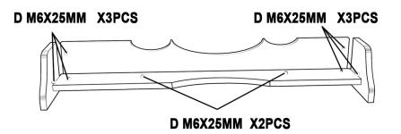
USE SCREWS (D) TO CONNECT BOARD (3) BOARD (4) AND BOARD (10) TOGETHER
