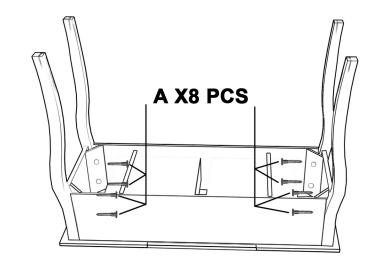
USE SCREWS (A) TO ATTACH THE TABLE BODY (11) TO THE TABLE LEGS(7)
