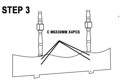
USE SCREW (C) TO CONNECT STEP2 WITH THE COMPLETED PART OF THE SECOND STEP
