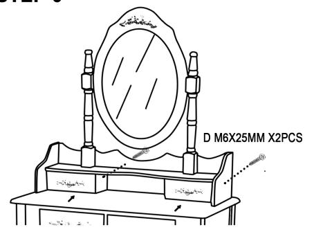
PLEASE THE SMALL DRAWER IN THE POSITION SHOWN AND ATTACH IT TO THE ASSEMBLED PART IN STEP 5 WITH THE SCREW (D)
