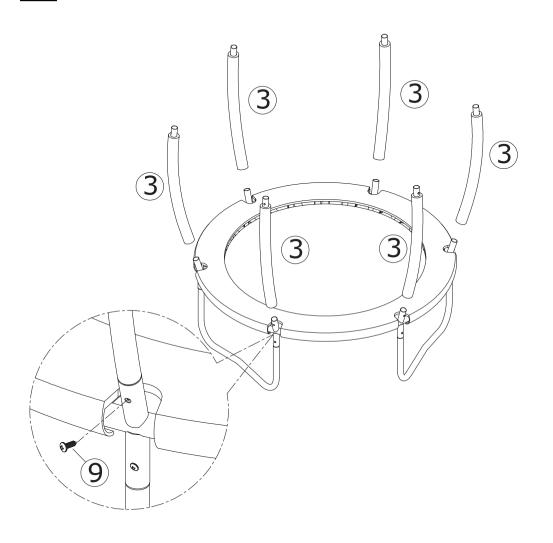
Connect the lower pole tubes and trampoline with screws.
