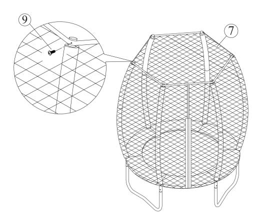
Attach the net to the upper pole tubes with screws.
