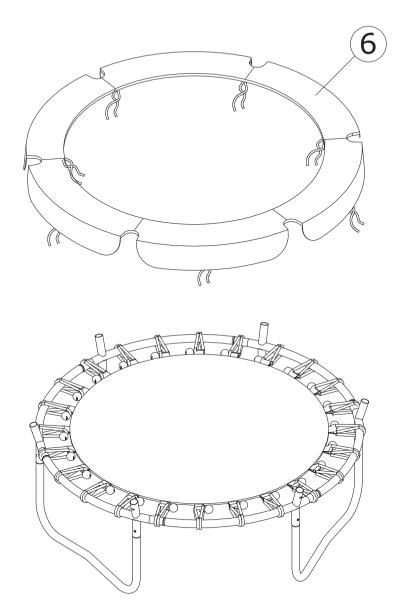
Lay the Frame Pad over the trampoline so that the bungee cords and the steel frame is covered.
