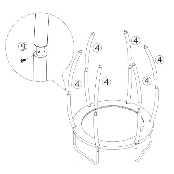
Connect the lower pole tubes and upper pole tubes with screws.
