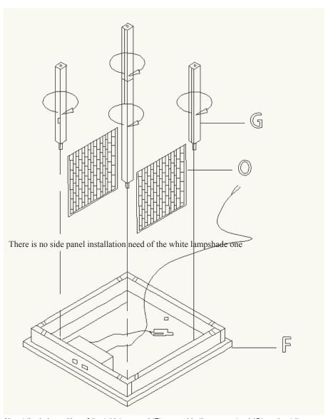
Aim at the hole position of the tabletop panel (F), assemble the upper stand (G), and put the side panel (O) into it along the pull groove.
