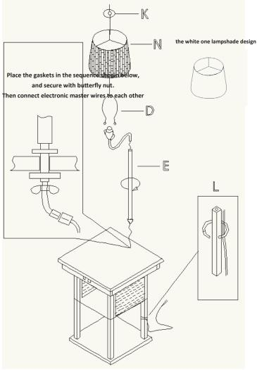
After assembling the iron tube, lock the lamp bracket to the lamp holder, and then lock the lampshade to the lamp bracket with the decorative round head nut (K). Finally, fix wire to the lower stand (I) with Velcro magic (L).
