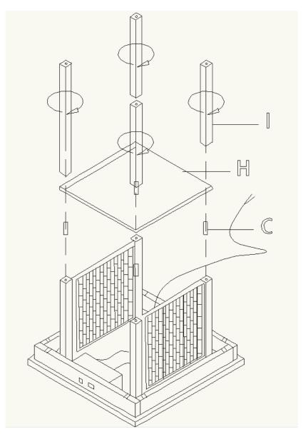
Connect the middle middle shelf panel (H) to the upper stand (G) with the double-headed screw (C), then assemble the lower stand (I).
