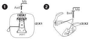
Please do not tighten the screws until all the screws are lined with holes. Try to tighten all the screws loosely initially and then tightly a little bit more. Do not over tighten a single screw as it will cause other screws hardly to be tightened. Tighten all the screws firmly in the end.
