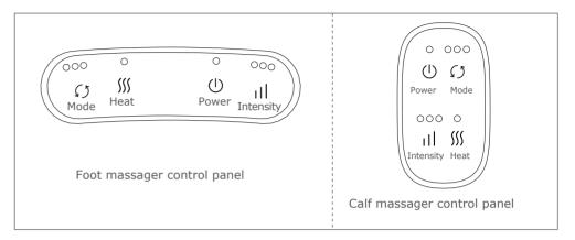
There is a control panel in the upper and lower sections of this product. It can be controlled separately when used separately, and any control panel can be controlled when used together, and the functions are synchronized.
