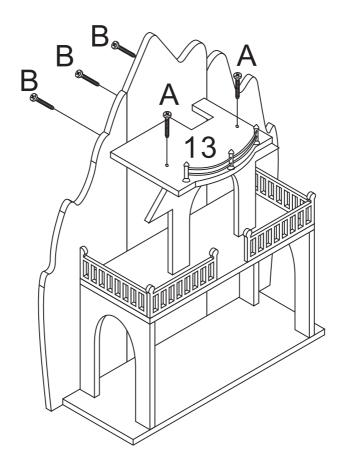
STEP 8: Assemble No.14,15 to No.9 with screws A.
