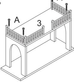
STEP 4: Assemble No.9 to No.3 with screws A.
