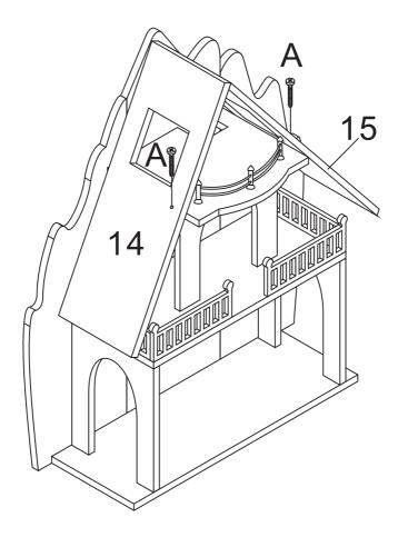
STEP 9: Assemble No.16 to No.14,15 with screws A.
