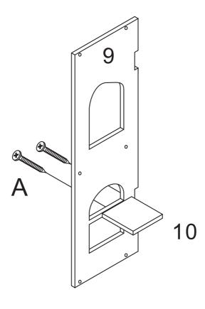
STEP 5: Assemble Part.9 to Part.3,4,5 with screws A.
