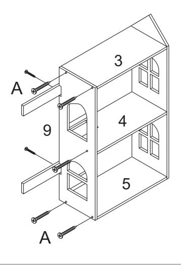
STEP 6: Attach Part.12 to Part.13 with dowel E, then assemble it to Part.9 with screws A.
