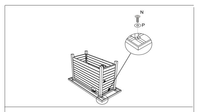
3.Attach the assembled base to the bottom of top using 4pcs of screws (N), and 4pcs M6 washers(P), make sure the panel (K) faces the valve stem.
