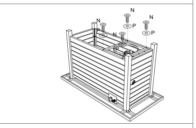
4. Connect the tank holder/base (I) With table legs(A/B/C) by 4pcs screws (N) and 4pcs M6 washers(P). Tighten all screws.
