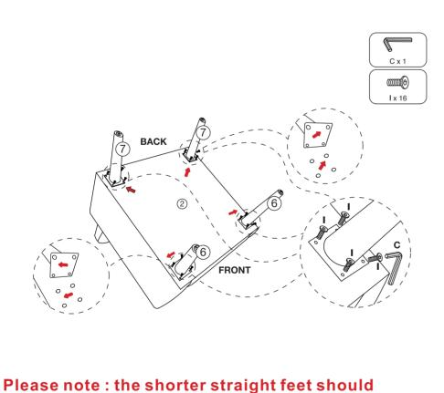
be attached to the front of the seat, while the high end of the angled feet should be attached to the front of the seat. Assemble according to the direction indicated by
