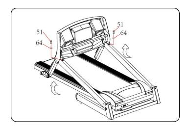
1. Holding the computer frame and uprights, unscrew bolt M8\*16(51) and lock washer (64) off right uprights, use the 5# Allen wrench to lock the computer and upright tube tight by screw M8\*16(51) and lock washer (64)
