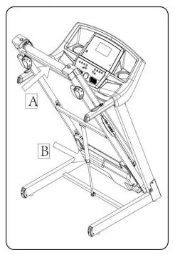
Pull up the base frame at position A, till hearing the sound that the air pressure bar B is locked into the round tube
