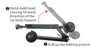
Step 2: Press the folding quick release wrench.
