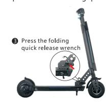
**Step 3:** Open the quick release wrench, unfold the handlebar stem towards both sides, insert the handlebar toward the center, and compress the quick release wrench.
