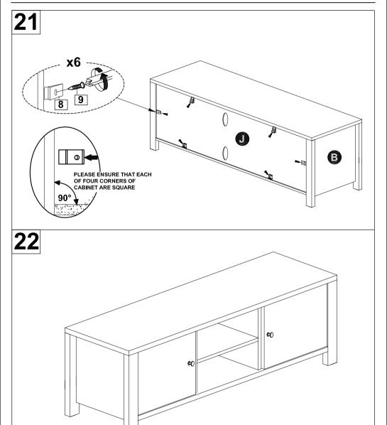
NOTE: THE MAXIMUM WEIGHT ON TOP PANEL IS UP TO 50KGS, AND ON PER SHLEF IS UP TO 5KGS.
