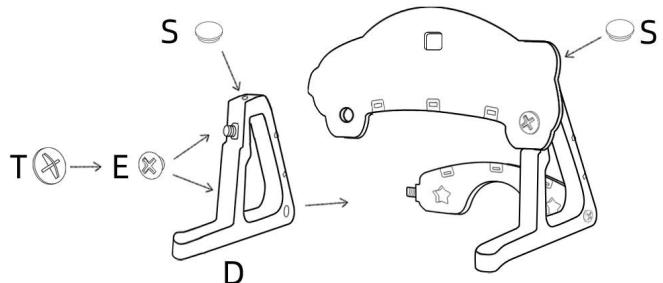
2. Use part S to cover the hole on the top of Part D (water or sand can be injected to stabilize the base)
