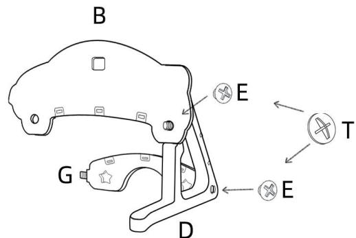
1. Use the screw knob tool part T to connect part B and D and part G through part E to build the basket base.
