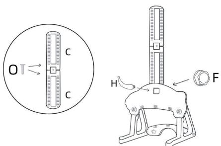
3. Connect two pieces of Part C using screw Part O, and use the screw part F to assemble the ring toss game hook part H the screw part F to assemble the ring toss game hook part H and fix part C.
