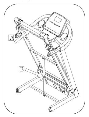
Pull up the base frame at position (A) till hearing the sound that the air pressure bar (B) is locked into the round tube.
