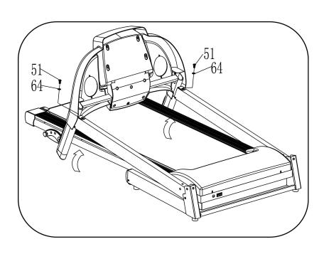
1. Hold on the Computer frame and use the 5# Allen wrench(12), M8\*20 bolt(51) and lock washer (64), fix the computer frame onto the right and left upright. Left picture for reference.
