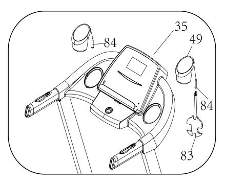
1.Put the Bottle cage (49) into the hole of the computer. Then use wrench with screw driver (83) and Bolt(84) to lock the bottle cage on computer(35). Left is same as right side.
