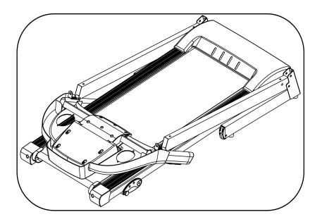
1. Open the carton, take out the above spare parts, put the Main Frame on the level ground.
