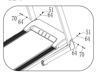
1. Use 5# Allen wrench, firstly lock upright onto base frame by bolt M8\*40 (70) and lock washer (64), then lock upright onto base frame by bolt M8\*20 (51) and lock washer (64).
