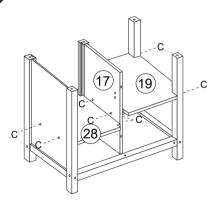
Assemble the panel No.17,18,19,28 with screws C
