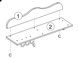
Assemble the panel No. 1, 2 with screws C
