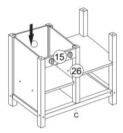
Attach the parts of step 6 to the part assembly of step 13 with screw C
