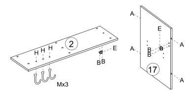
Assemble the part M to the panel No. 2 with screws H, and the part E to the panel No.2,17with screws B, then insert the wooden plug A into the panel No.17
