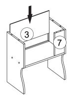
Insert the panel No.3 between the panels No.4 and No.6,and assemble the panel No.7 to No.5 with wooden plug A
