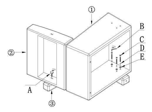
**Note:** The three bolts of the bottom frame can't be tightened at one time. After the back rest and armrest are connected with bolts, they can be tightened uniformly.
