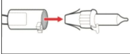
Release the latch located on the side of the bulb.
