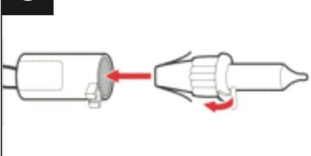
Insert a new bulb and lock the latch.
