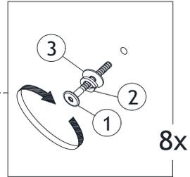
Do not tighten the hardware completely!
