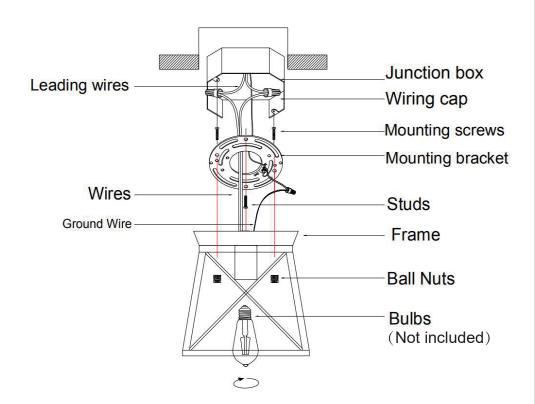
Read instructions carefully and turn electricity off at main circuit breaker panel before beginning installation.
