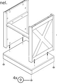
6-Install the top support on the top panel, and install the top on the side 5 panel.
