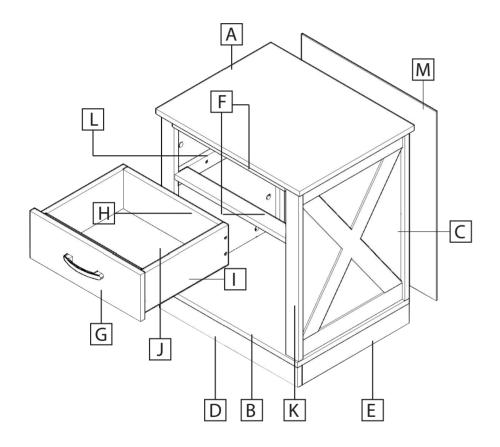
1-Assemble the drawer side panel and drawer back panel. Install the bottom panel and attach the drawer slide at side panel. Then assemble the drawer handle with screws.
