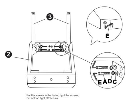
COSTWAY www.costway.com PRODUCT ASSEMBLY STEP 2 Put the screws in the holes, tight the screws, but not too tight, 90% is ok.
