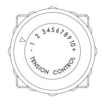
Ten level tension control: The user can adjust the damping to take exercise freely. This item has ten level tension control (1~10) and damping (1 is minimum, 10 is maximum)
