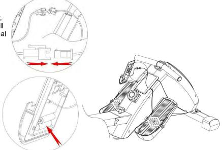
Open the computer and Install the battery .See the right picture.
