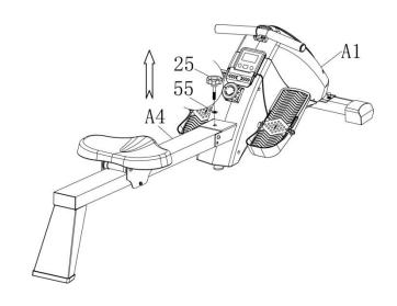
2. Unscrew the plum knob(25) from the Main frame(A4) and remove the Washer(55).
