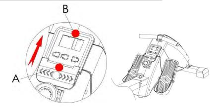
After unpacking the computer, note the signal line head. Install the battery and check if the signal cable plug is on the right plug direction before install the computer back.see the picture
