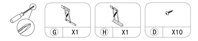
Assemble the installed G and H with No. 1 panel with Screw D.
