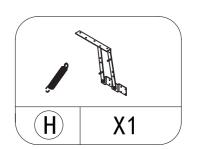
EN: Assemble the springs and the raise handles together in G and H.
