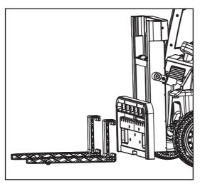
11. Battery bin circuit connection Connect the power cord plug with the battery plug, please note that red is connected to red and black is connected to black.
