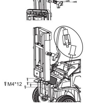
9. Install the front fork guardrail, put the front fork guardrail into the central box of the front fork lifting assembly from front to back, and fix it with screws.
