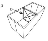
Fix the metal support frame (D) in the middle
