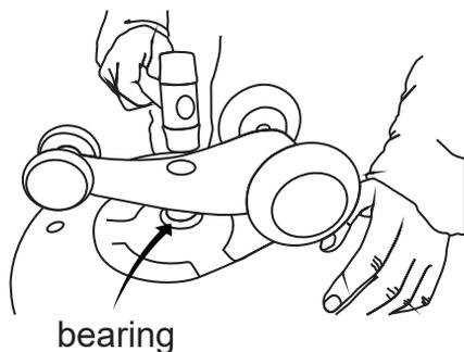
4. As shown in picture, check if the button of the wheel is installed in right place, make sure this button reaches the bottom.
