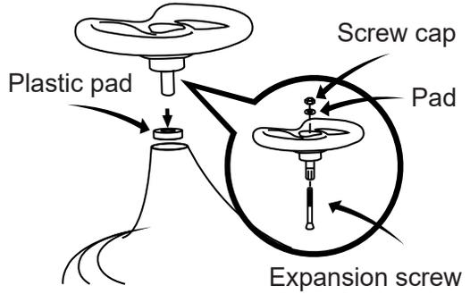
8. As shown in picture, adjust the steering wheel to make the notched end of the steering wheel face forward.
