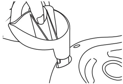
6. As shown in picture, knock at the bottom of the rear wheel mechanism by a rubber hammer, make the bearing of the rear wheel mechanism insert into the hole of the swing car body totally.
