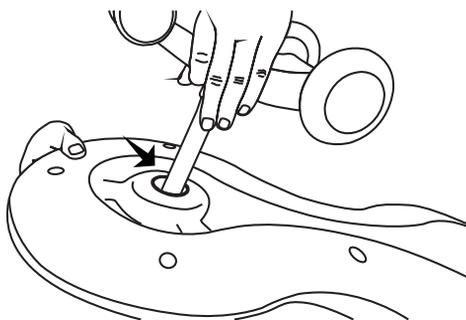
3. As shown in picture, knock at the bottom of the front wheel mechanism by a rubber hammer, and fully insert the bearing of the front wheel mechanism into the hole of the swing car body.
