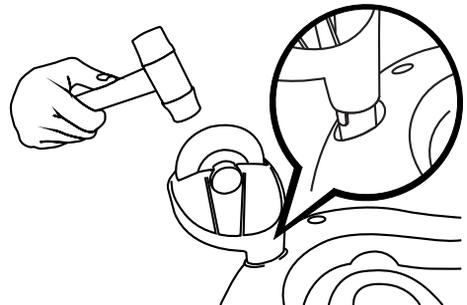
7. Take out the steering wheel, check if the expansion screw is loose, put PP bearing into the holder of the body.
